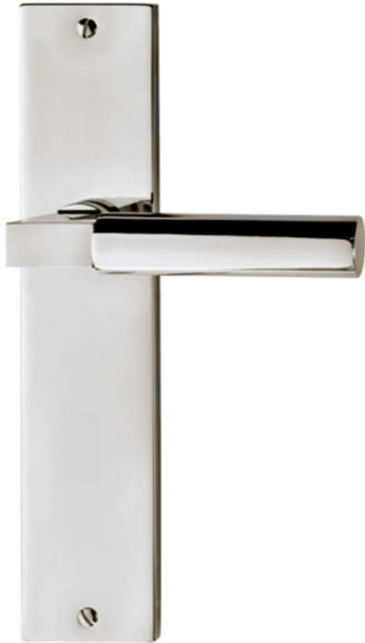
LEVER #14.964.266 set with escutcheon "BAUHAUS" Escutcheon #14.J964 236 x 48 x 7 mm Polished Chrome Plated Brass Plated.
