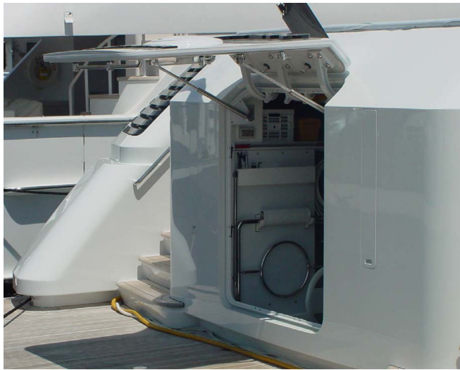
Application: Two 22-38-400 gas springs, 2342 Newton force each with custom made brackets.
