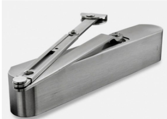
#35.083H Hydraulic door closer for fire rated full size doors; - Force 7 Finish: Satin Stainless Steel or Polished Stainless Steel cover with STEEL arm and bracket
