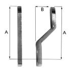
Cams: #115.85 straight #115.87 bend; dimension A= 2 3/8 inch dimension B= 3/4 inch
