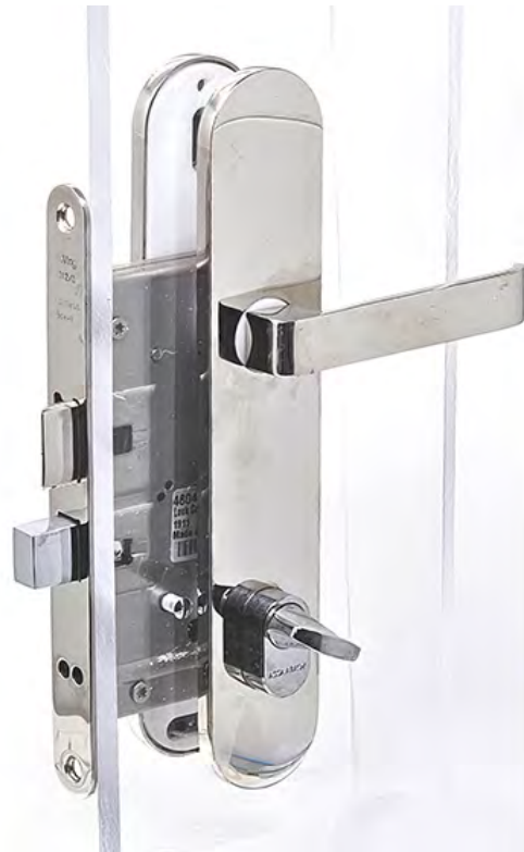
#11.SEFT.019 Entry Mortise Lock. Set 55 mm backset. Heavy Duty. Solid Latch. Mega Yacht Upgrade. Polished Stainless Steel
