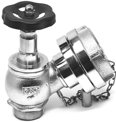
#91.778 Valve + 1 1/2" with N=66 Storz Coupling and Dust cap Steel powder coated turning wheel Thread: 1 1/2" BSP. Valve chrome over brass
