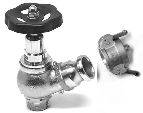
#91.075 Valve 1 inch showing with Stainless Steel Camlock Coupling & cap Steel powder coated turning wheel Thread: 1" BSP. Valve chrome plated brass
