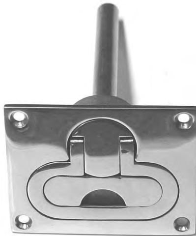
Hatch Pull with locking cam #43.219; 316 Stainless, face plate: 3 3/4 x 3 inch; length shaft: 5 1/8" diameter: 1/2"
