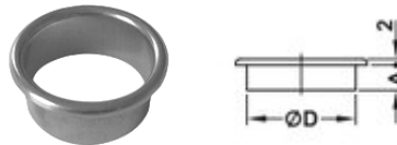
#21.2801 Brass #21.2701 nickel Brass Cover ring for hole in door: Drill 35 mm hole; D = 35 mm; A = 19 mm
