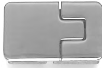
Hatch hinge #42.894, "2 x 4" heavy duty, with 100 degree backstop, no screws showing. Size: 4 3/8" x 2 5/16" x 5/8" (sizes and drawing on page 4-2-0-A)
