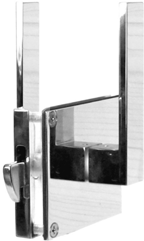
#81.8808 Glass or Wood Sliding Rim lock w. Strike Box. 1/4 to 1/2 inch thick glass and up to 3/4 inch wood. Chrome Plated Brass
